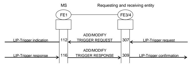
Figure 5.11: MS receiving trigger definitions and rejecting triggers
