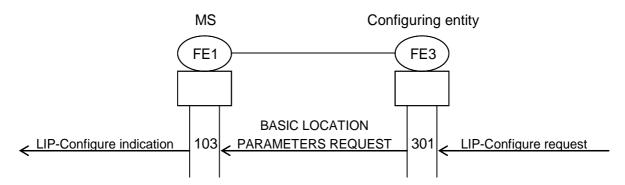
Figure 5.3: MS receiving basic parameters
